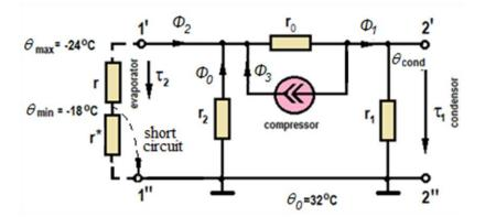
Figure 4: U-shaped electrical substitution scheme of refrigerating machine
