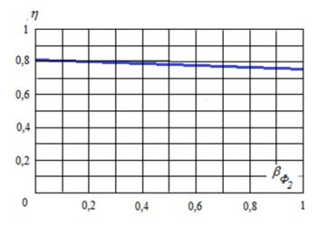
Figure 6: Refrigerating machine efficiency in relation to evaporator loading  $\eta = f(\beta_{\Phi_2})$
