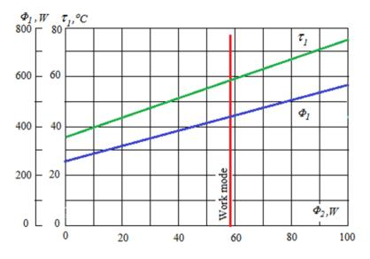
Figure 5: Loading parameters of household refrigerator refrigerating machine  $\tau_1 = f(\Phi_2)$  and  $\Phi_1 = f(\Phi_2)$
