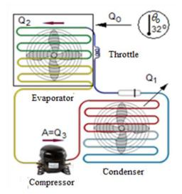
Figure 1: One contour piping system for the refrigerator unit
