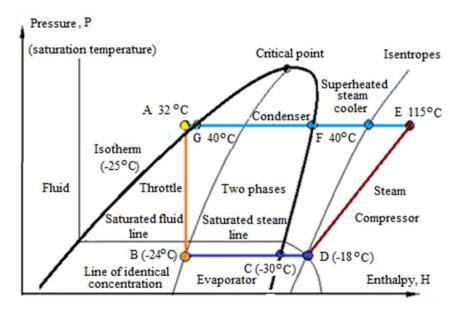
Figure 2: Diagram pressure - enthalpy
