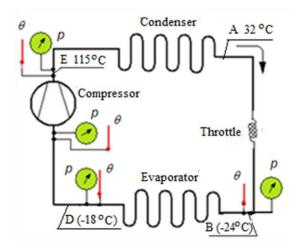
Figure 3: Schematic diagram of the compressor refrigeration performance testing under the simplified methodology
