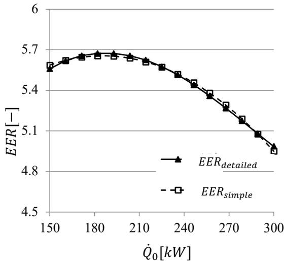
**Figure 7: EER values obtained from detailed and simplified model as a function of the cooling capacity**
