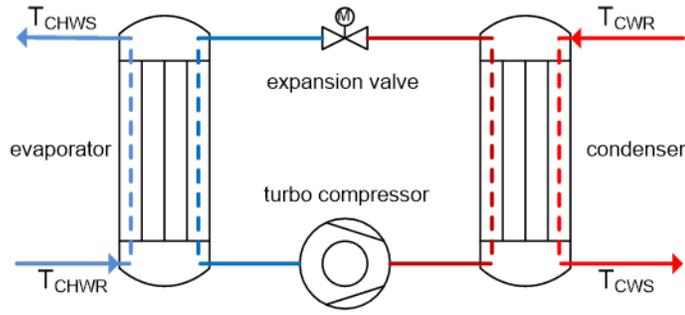
Figure 2: Scheme of a water cooled turbo compressor chiller
