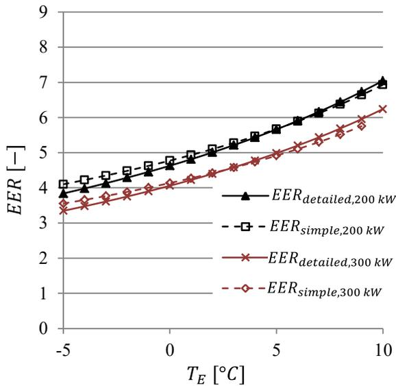
**Figure 3: Comparison of EER values obtained from detailed and simple model at varying evaporation temperatures**
