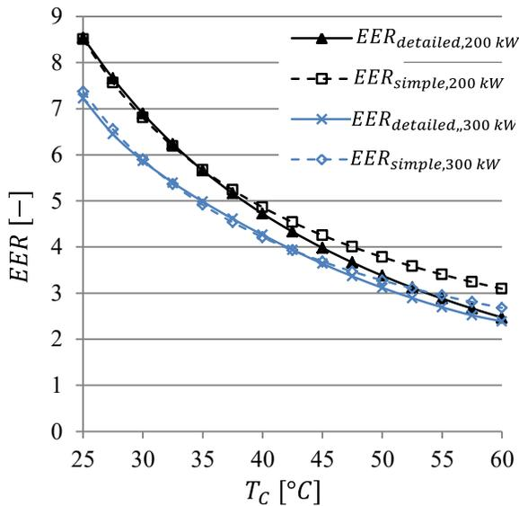
**Figure 5: Comparison of EER values obtained from detailed and simple model at varying condensation temperatures**
