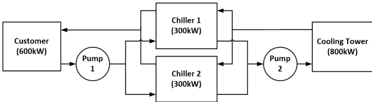
Figure 1: Example of examined refrigeration system
